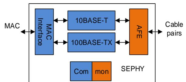
Figure 1: SEPHY block diagram
