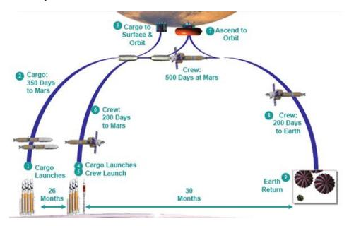
Figure 2. NASA Design Reference Architecture 5.0 for manned missions to Mars.<sup>4</sup>
