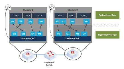
Figure 4. Relationship between network-level and system-level tools.
