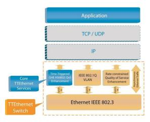
Figure 1. TTEthernet QoS in the OSI model.
